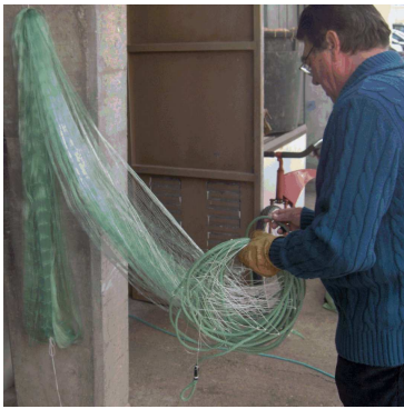
Mounting float cord on a 50-mesh lemon / dover sole net
